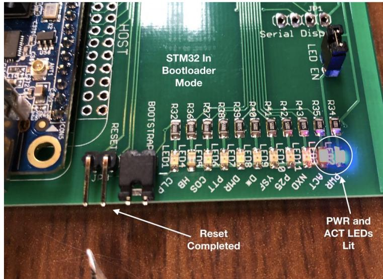
After the STM32F446RET6 enters bootloader mode, send the following command at the NaoPi NEO's shell prompt:
