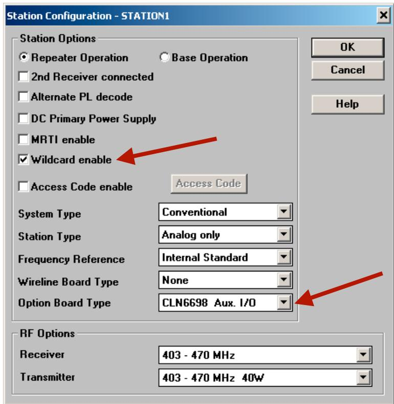
The MTR2000 SCM communicates with station modules (including the CLN6698 Auxiliary I/O board) via a Serial Peripheral Interface (SPI) synchronous serial bus operating in SPI mode 3 with 16 bit datagrams. The original CLN6698 exposed two separate SPI “slaves” to the bus, one for the inputs and one for the outputs. In each case, two 8-bit shift registers connected in series forms the hardware interface to convert parallel I/O (GPIO lines) to serial data on the SPI bus.
