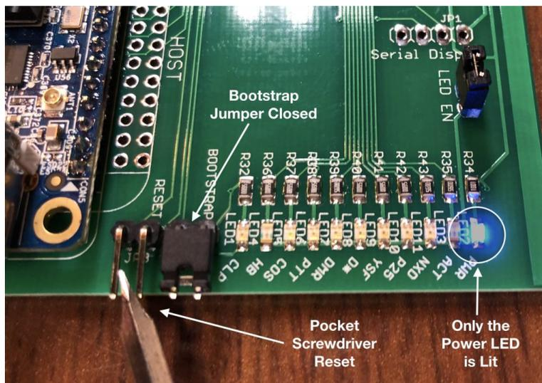
Note that while the board is being reset only the Power LED should be illuminated. Once the board has successfully been reset and is in bootstrap mode, the Power and Activity lights will remain lit constantly. Actually, the DMR and COR LEDs are also lit very dimly; it may not be possible to see them lit at all in a well lighted room.
