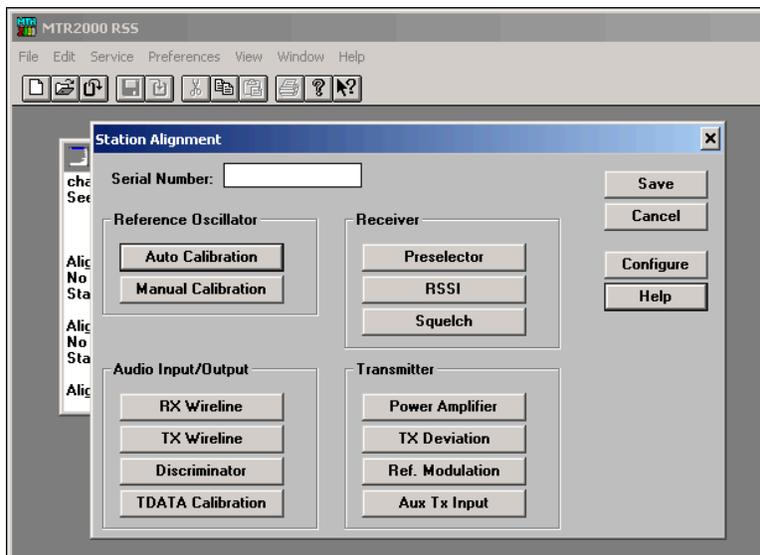
STM32-DVM-MTR2K analog conditioning circuitry is optimized for the MTR2000, which makes alignment very simple. With no input signal present, the MTR2000 Discriminator output level should
