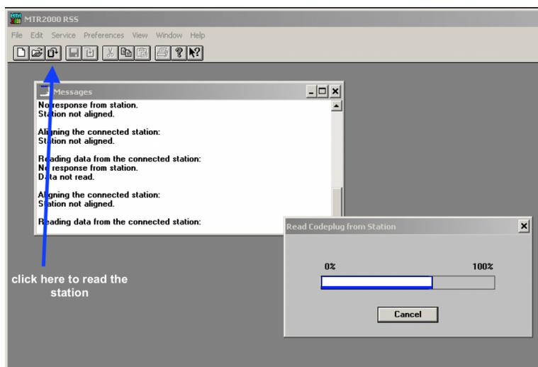
There are two items that must be set: “Aux Tx Audio Control” and “External PTT Mapping”. Once the station is read, a new “Station Configuration” window will appear, and a new menu item called “Personality” will show up between “Edit” and “Service” in the RSS menu bar. The personality menu is only present when a Station Configuration window is active.
