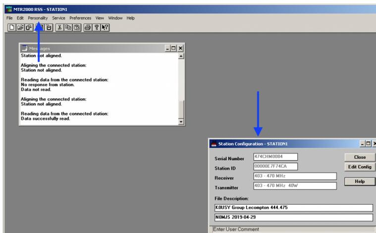
Under the “Personality” menu, select “Channel Information”. A new window will appear. In the upper left area of the window is a section box marked “Option”. From this list we’ll be working with the “Audio” and “PTT” menus. In the Audio settings, “Aux Tx Audio Control” must be set to the “Flat”. This directs the station to NOT pre-emphasize or limit the Aux Tx Audio input.
